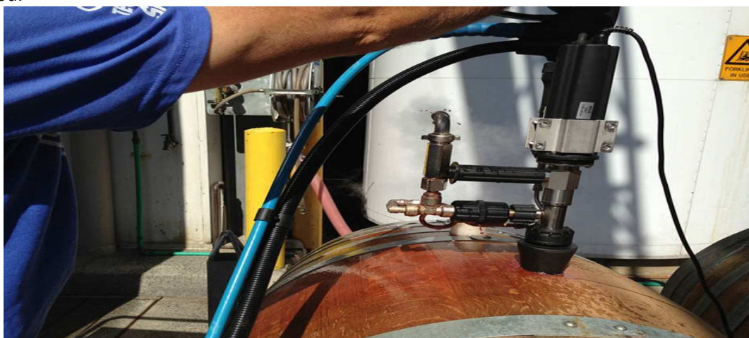
Wine Barrel Cleaning Dry Steam Machine
