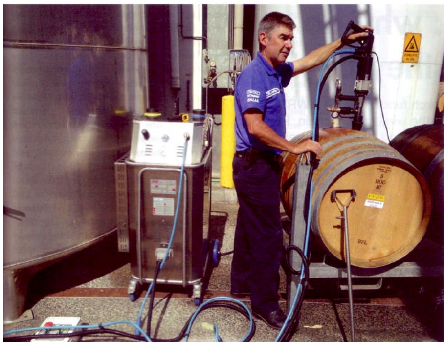
Duplex director Murray McDonald providing a wine barrel cleaning demonstration in the Yarra Valley of the Bacchus steam pressure machine.
