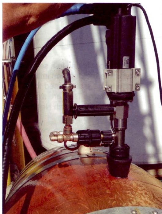
The Bacchus steam pressure machine's diffuser inserted into a wine barrel.
