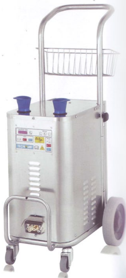
The Bacchus dynamic is a mono-phase or three-phase steam generator with an automatic refilling system. It was among the machines demonstrated at Sticks Winery in the Yarra Valley last month.
