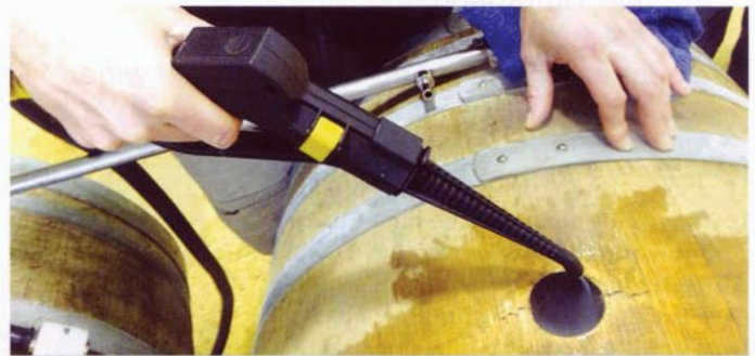
All steamed up: A Wine Barrel Company unit gives a bung hole a high-temperature overhaul and the overall clean will extend the life of an average wine barrel.
